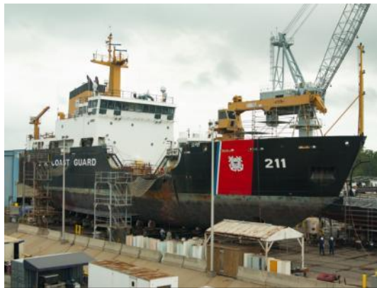
WLB 211 (OAK) is the first of sixteen 225' Seagoing Buoy Tenders to undergo a Midlife Maintenance Availability at the Coast Guard Yard. Coast Guard photo.
