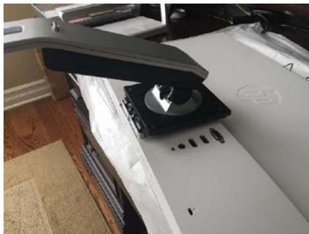
The picture reproduced above shows the bottom tabs of the VESA mount adapter bracket inserted into slots in the back of a video monitor. *See* Ex. 1003, 6.
