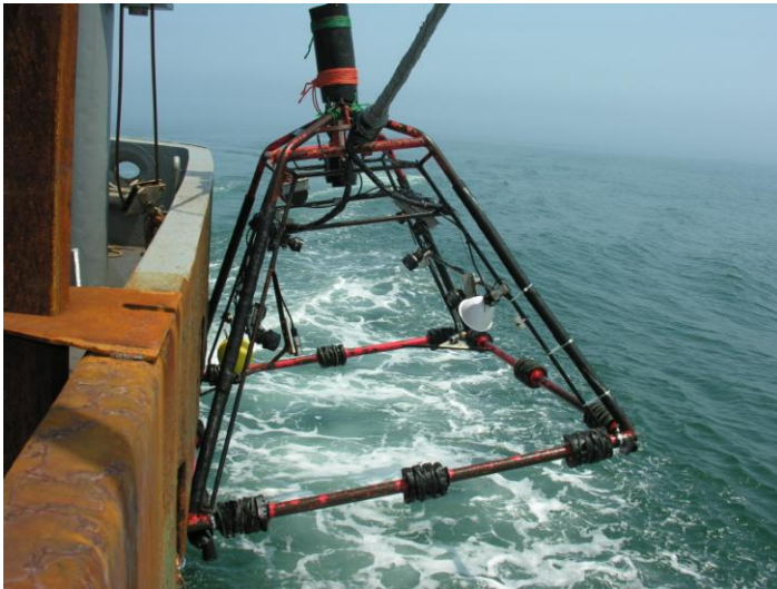
Figure 4. The SMAST video sampling pyramid mounted on the side of a commercial fishing vessel.
