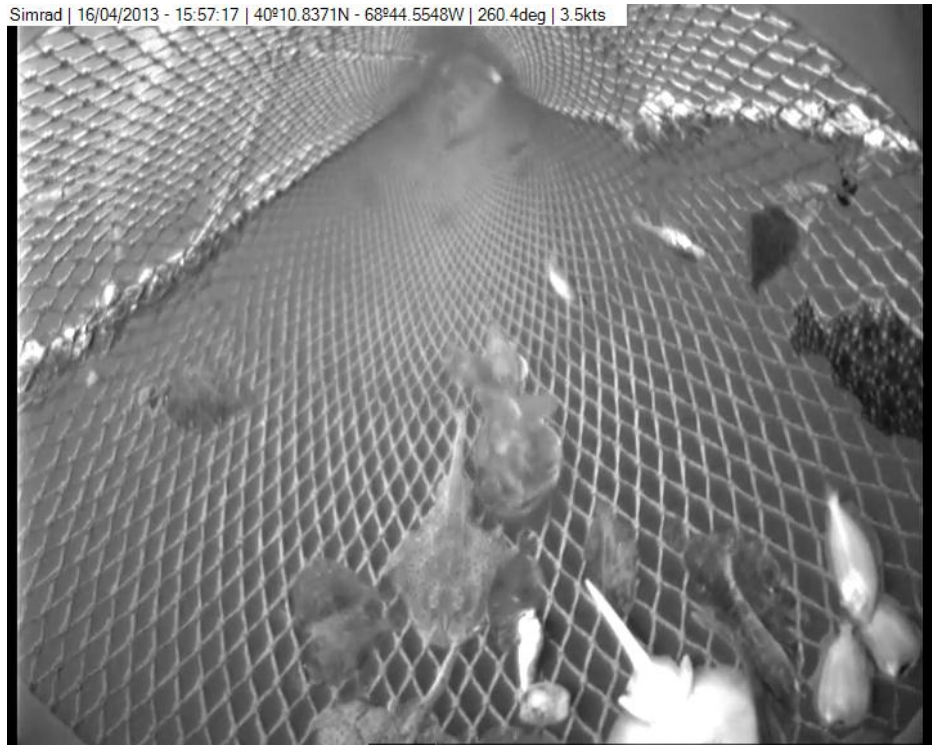
Figure 7. A Digital image of groundfish from a test system that may allow the sampling of fish as they pass through and then exit the net without damaging them.
