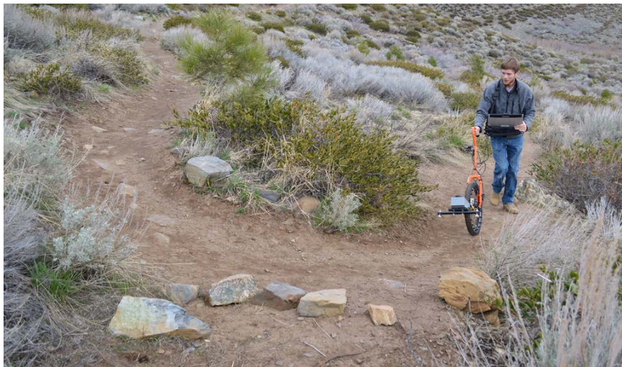
A High Efficiency Trail Assessment Process, or “HETAP,” is a wheeled piece of technology that is used to collect objective data on trail-accessibility standards such as slope and grade. Source: Beneficial Designs, no date.
