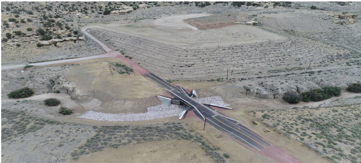
Residential and grazing areas near the Quivira mine, where EPA by 2018 removed contaminated soil and temporarily covered and stabilized a waste pile, with work by Arrow Indian Contractors, a Navajo-owned company. EPA also repaired roads, culverts, and a bridge as needed to enable cleanup.
