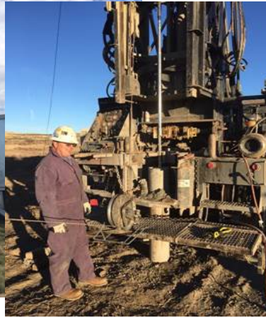
Sonic drilling used to conduct sampling during the groundwater investigation.
