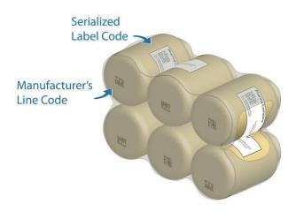
Immediately after the serialized label is applied to the unit, custom inspection equipment would synchronize the label with the manufacturer's line code. The units would travel down the packaging line with two unique codes towards a bundling station, which would group and shrink wrap several units into small bundles. A labeling station would apply a unique serialized label to the bundle.
