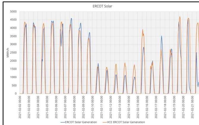
Figure 4.13: ERCOT solar generation provided by the EIA Hourly Electric Grid Monitor (blue) and ERCOT solar generation as calculated by the VCE weather datasets (orange). This is plotted from February 2<sup>nd</sup> 2021 through February 21<sup>st</sup>, 2021. The time zone is set to EST.
