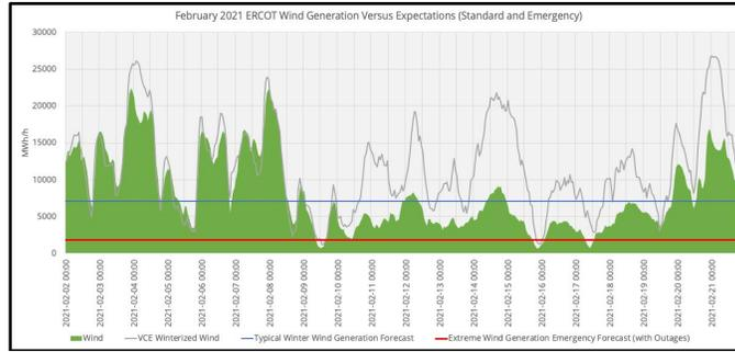
Figure 2.10: ERCOT wind generation (green) alongside various wind capacity expectations ERCOT had for normal winter peak (blue) and extreme low wind capacity expectations (red). The gray line is the VCE derived wind power production with standard turbine winterization (less impact from icing). This is plotted from February 2<sup>nd</sup> 2021 through February 21<sup>st</sup> 2021. The time zone is set to EST.
