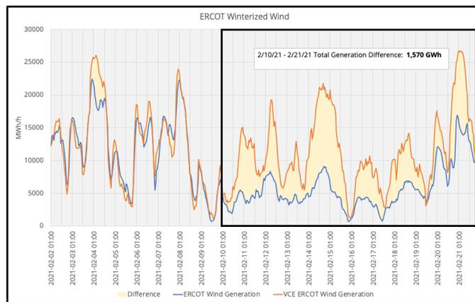
Figure 4.2: ERCOT wind generation provided by the EIA Hourly Electric Grid Monitor (blue), ERCOT wind generation as calculated by the VCE weather datasets (orange) and the difference between the two datasets (cream). This is plotted from February 2<sup>nd</sup>, 2021 through February 21<sup>st</sup>, 2021.
