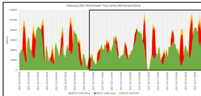
Figure 6.1: ERCOT wind generation as calculated by the VCE weather datasets (green), ERCOT utility solar generation as calculated by the VCE weather datasets (red) and ERCOT distributed solar generation as calculated by the VCE weather datasets (orange). This is plotted for weather from February 2<sup>nd</sup>, 2021 through February 21<sup>st</sup>, 2021 with assets from a hypothetical 2050 clean energy grid WIS:dom-P scenario.
