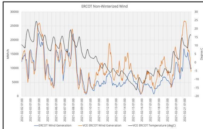
Figure 4.3: ERCOT wind generation provided by EIA's Hourly Electric Grid Monitor (blue), ERCOT wind generation with more stringent icing as calculated by VCE's weather datasets (orange) and average wind farm hub height temperature from VCE's weather datasets (black). This is plotted from February 2<sup>nd</sup>, 2021 through February 21<sup>st</sup>, 2021.
