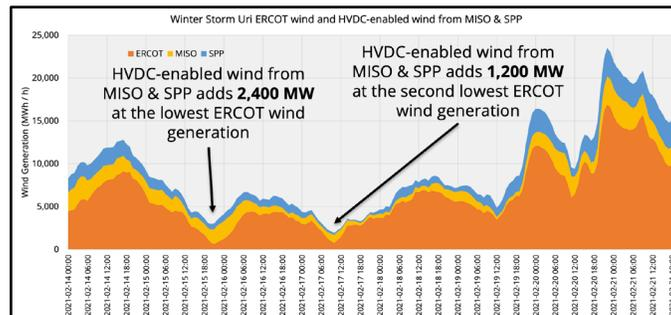
Figure 4.11: The wind power that the HVDC transmission lines could add to ERCOT from MISO (yellow) and SPP (blue). These are stacked upon the ERCOT local generation from wind. These values are scaled from the actual production reported in each RTO. The time zone is set to EST.
