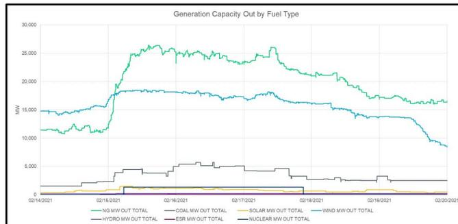
Figure 2.6: ERCOT created graphic from an emergency board of directors meeting which shows the outage capacity outages by fuel type.
