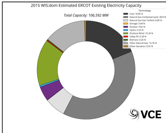
Figure 2.3: WIS:dom estimated installed capacity for ERCOT at the end of 2015. The total capacity modeled for this region is 106.6 GW.
