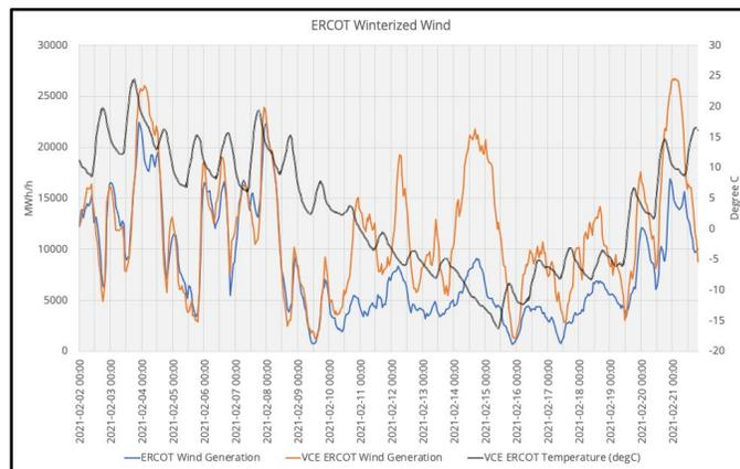
Figure 4.1: ERCOT wind generation provided by the EIA Hourly Electric Grid Monitor (blue), ERCOT wind generation as calculated by the VCE weather datasets (orange) and average wind farm hub height temperature from the VCE weather datasets (black). This is plotted from February 2<sup>nd</sup> 2021 through February 21<sup>st</sup> 2021. The time zone is set to EST.
