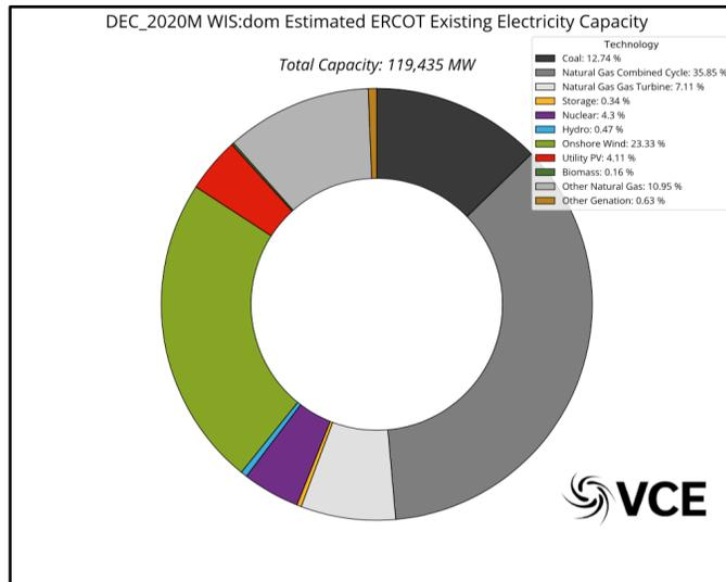
Figure 2.2: WIS:dom estimated installed capacity for ERCOT as of December 2020. The total capacity modeled for this region is 119.4 GW.
