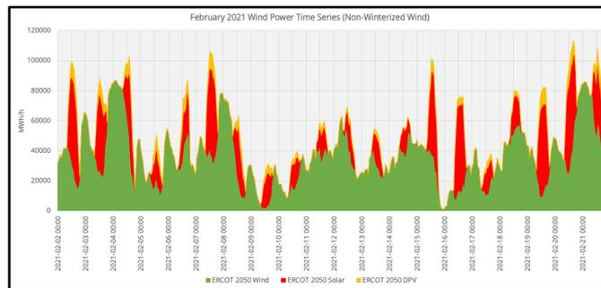
Figure 6.2: ERCOT wind (green), utility solar (red), and distributed solar generation (orange) as calculated by the VCE weather datasets. This is plotted from February 2<sup>nd</sup>, 2021 through February 21<sup>st</sup>, 2021 for a hypothetical clean energy grid scenario from a 2050 WIS:dom-P model run.
