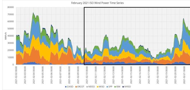
Figure 4.8: ISO wind power generation provided by the EIA Hourly Electric Grid Monitor for all ISOs across the contiguous US. This is plotted from February 2<sup>nd</sup>, 2021 through February 21<sup>st</sup> is highlighted in black to point out the difficult period in ERCOT. The time zone is set to EST.
