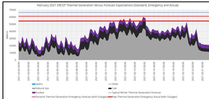
Figure 2.9: ERCOT thermal generation alongside various thermal capacity expectations ERCOT had for normal winter peak (blue), extreme thermal outage capacity expectations (red) and thermal outage expectations recalculated with thermal outages observed during the energy crisis (bold dark red). This is plotted from February 2<sup>nd</sup> 2021 through February 21<sup>st</sup> 2021. The time zone is set to EST.
