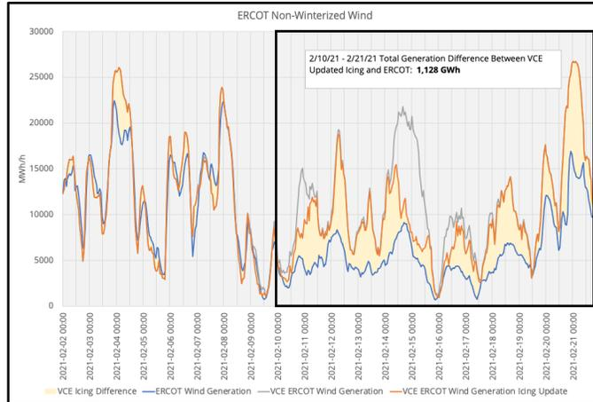
Figure 4.4: ERCOT wind generation provided by the EIA Hourly Electric Grid Monitor (blue), ERCOT wind generation as calculated by the VCE weather datasets with more stringent icing conditions (orange) and the difference between the two datasets (cream). The regular VCE ERCOT wind generation with typical icing criteria is plotted for comparison (gray). This is plotted from February 2<sup>nd</sup>, 2021 through February 21<sup>st</sup>, 2021.
