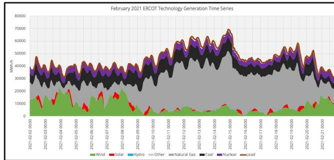
Figure 2.8: ERCOT generation by fuel type. Load is also plotted. This is plotted from February 2<sup>nd</sup> 2021 through February 21<sup>st</sup> 2021. The time zone is set to EST.
