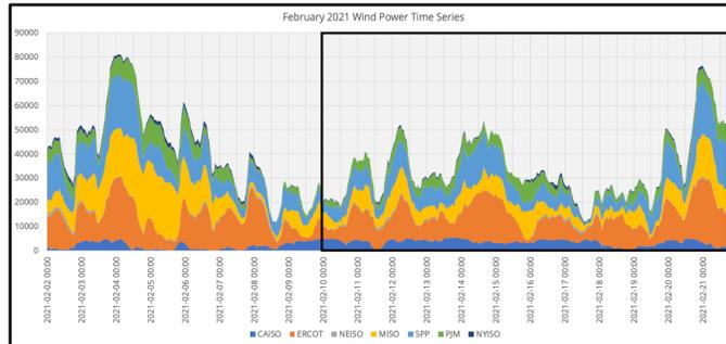
Figure 4.9: ISO wind power generation derived by VCE using standard icing criteria for all ISOs across the contiguous US. ERCOT is the bolded orange series. This is plotted from February 2<sup>nd</sup>, 2021 through February 21<sup>st</sup>, 2021. February 10<sup>th</sup> through 21<sup>st</sup> is highlighted in black to point out the difficult period in ERCOT. The time zone is set to EST.
