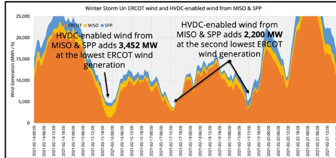
Figure 4.12: The wind power that the HVDC transmission lines could add to ERCOT from MISO (yellow) and SPP (blue). These are stacked upon the ERCOT local generation from wind. These values are scaled from the VCE winterized possible wind generation in each RTO. The time zone is set to EST.
