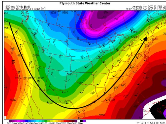
Figure 3.3: The mid-level (500 mb) contoured heights with wind speeds overlaid from Plymouth State Weather Center archives at 00 UTC on February 15<sup>th</sup>, 2021.
