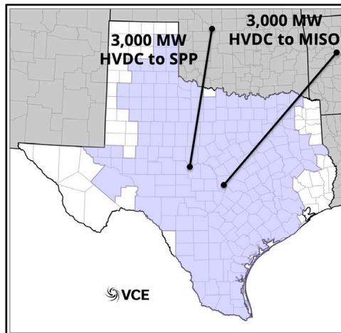
Figure 4.10: Illustration of two HVDC transmission lines connecting ERCOT with MISO and SPP. The connection points are illustrative and do not represent actual siting preferences.
