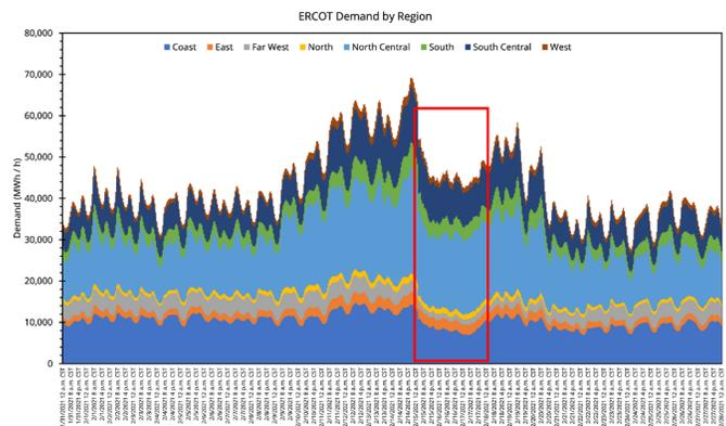
Figure 1.1: The electricity demand for the eight ERCOT regions. The rolling blackouts are highlighted in the red box. All regions appear impacted by the blackouts. Data is from the [EIA 930](#).
