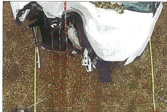
Figure 8: Top view of crush to front of case vehicle from impact with clump of trees, each increment on rods is 5 cm (2 in)
