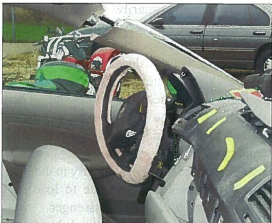
Figure 12: Right side view of deformation to steering wheel and steering column
