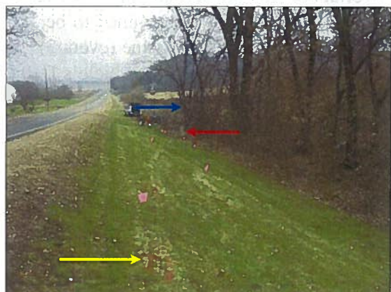
Figure 3: Vehicle touchdown location (yellow arrow) from vault and approach to telephone utility box impact (red arrow) and impact with clump of trees (blue arrow)
