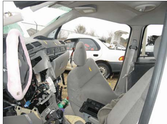
Figure 10: Left side view of steering wheel, instrument panel and displacement of front right seat back and head restraint due to the back right passenger loading the seat back into the front right passenger
