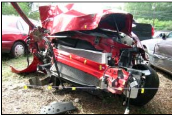
Figure 7. Damage from the 13 cm (5") tree.
