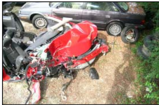
Figure 8. Overhead view of the damage from the 51 cm (20") tree.
