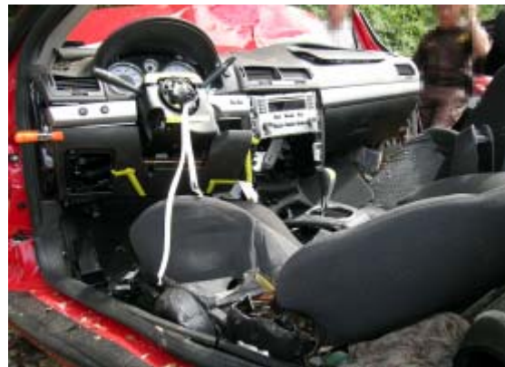
Figure 10. Driver contact to the knee bolster.
