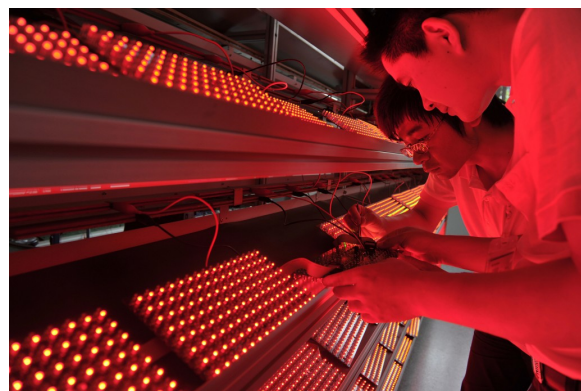
Employees measure the aging levels of low-energy consumption light bulbs at a factory in Nanjing, Jiangsu province, May 18, 2012. REUTERS/Sean Yong
