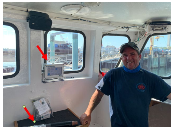
Figure 4. Dissolved oxygen sensor (lower red arrow) and deck display (upper red arrow) being used by New England lobstermen to track the onset of hypoxia on the East Coast (Photo credit: Lowell Instruments)
