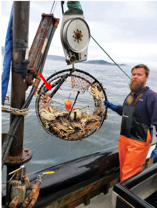
Figure 3. Commercial crabber bringing on deck a crab pot equipped with a smart dissolved oxygen sensor (red arrow) developed with support from NOAA NCCOS' Coastal Hypoxia Research Program. (Photo credit: Pat Kemmish, F/V Richard H.)
