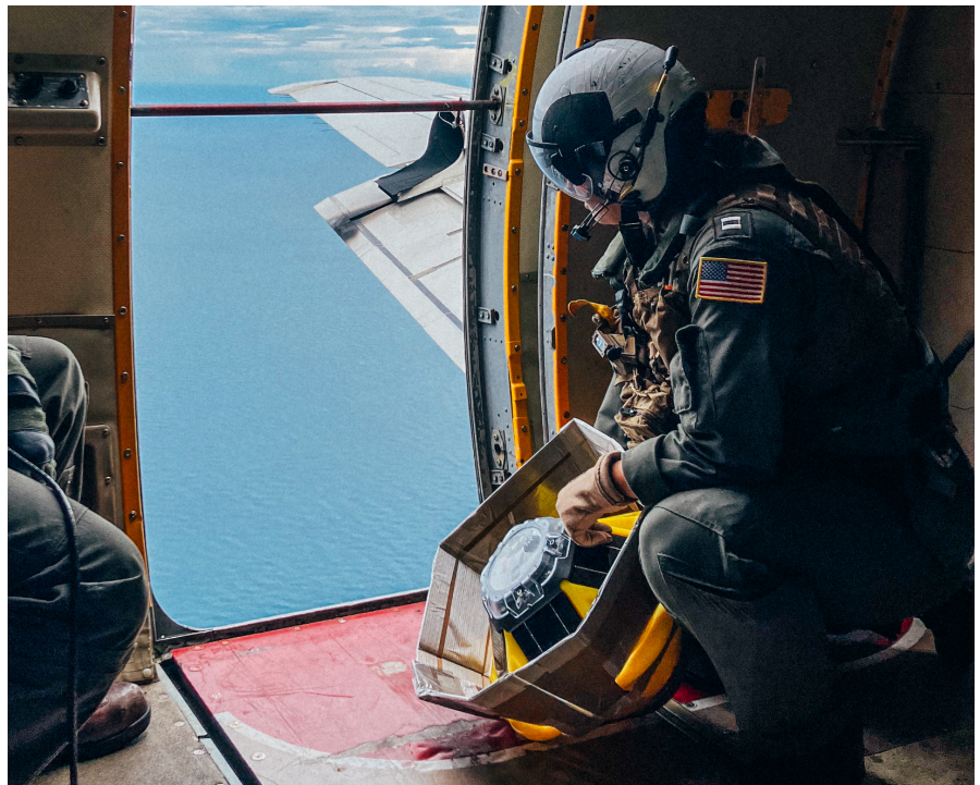
Figure 6: In partnership with the NOPP program, Sofar developed an air-deployable Spotter buoy, which has been deployed into hurricanes including 2024’s Hurricane Milton.
