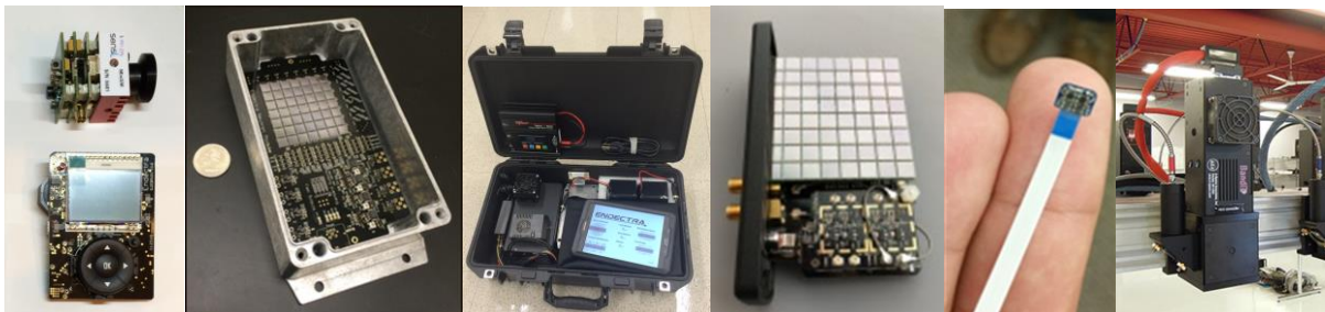
Fig 6. Endectra SBIR funded innovations, from Left to Right: (a) Endectra CBSG-2 (Cerenkov Borosilicate Glass) prototype neutron detector (Aug 2015); (b) CBSG-3 neutron detector module (Jun 2016); (c) Tri-Modal (gamma, fast neutron, slow neutron) Radioisotope Identification Device incorporating Endectra and H3D technology (Aug 2016); (d) CBSG-4 wireless radiation sensor network module (Feb 2017); (e) CMSI probe utilized in arrays of multiple on-skin probes for radiotherapy (Dec 2017); (f) Online metrology tool within which we helped integrate a SiPM-based spectrometer for a leading domestic photovoltaic manufacturer (July 2018).
