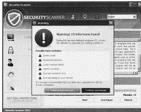
Fig. 2. An example of Scareware. The pop-ups proclaim that the victim's computer is infected, and often cannot be closed.
