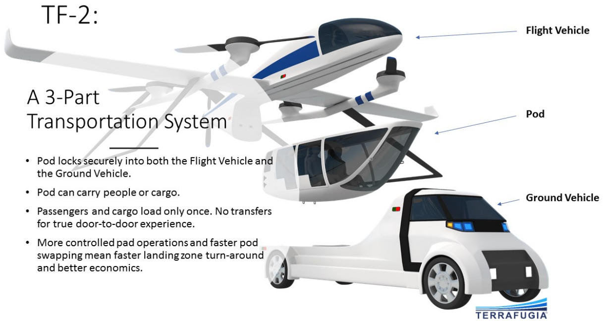
Figure 3: The TF-2 three-part transportation system
