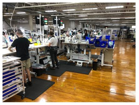
All the equipment is at standup stations, since the sewers move from machine to machine as they make each garment.
