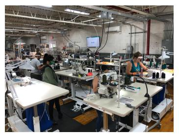
In a lean methodology, the sewer makes one perfect shirt, and then makes another. The sewing machines are typically arranged in a "U" so that the garment begins at the first machine, and then is taken by the sewer to the next machine, and so on until the garment is complete at the last machine.
