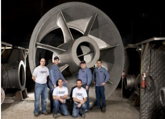
ST. MARYS TEAM MEMBERS STAND IN FRONT OF A 27-TON DIFFUSER CASTING WHICH IS NOW PART OF THE WORLD'S LARGEST PUMP STATION BUILT IN NEW ORLEANS, LA BY THE U.S. ARMY CORPS OF ENGINEERS. THE DIFFUSERS CAN HANDLE A PUMPING RATE OF 150,000 GALLONS OF WATER PER SECOND.
