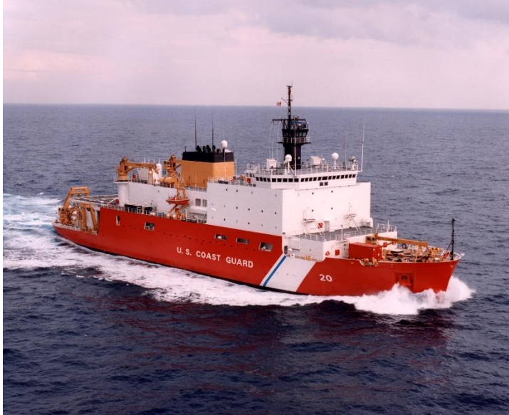
Figure 3. Coast Guard Cutter Healy, a 420-foot medium endurance icebreaker/research vessel, is the only icebreaker currently dedicated to Arctic operations. No other U.S. military service branch operates icebreakers. 57
