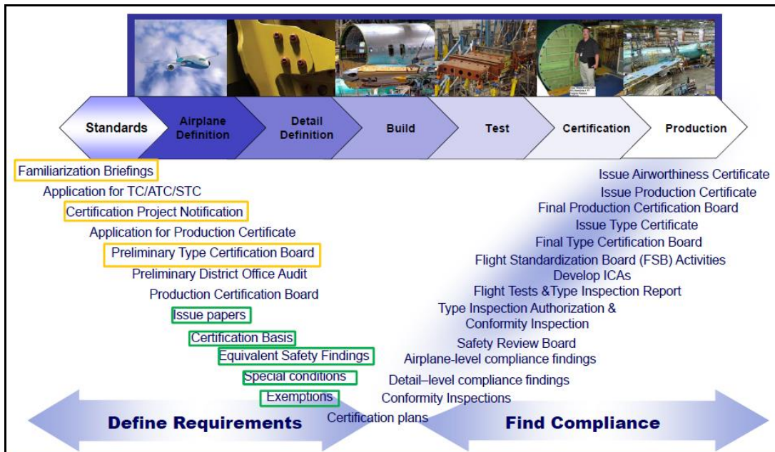
Figure 3 Diagram of FAA Certification Process
