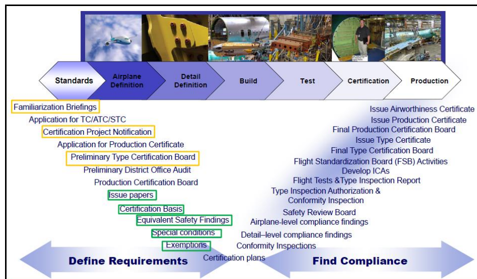
Figure 45: Diagram of FAA Certification Process
