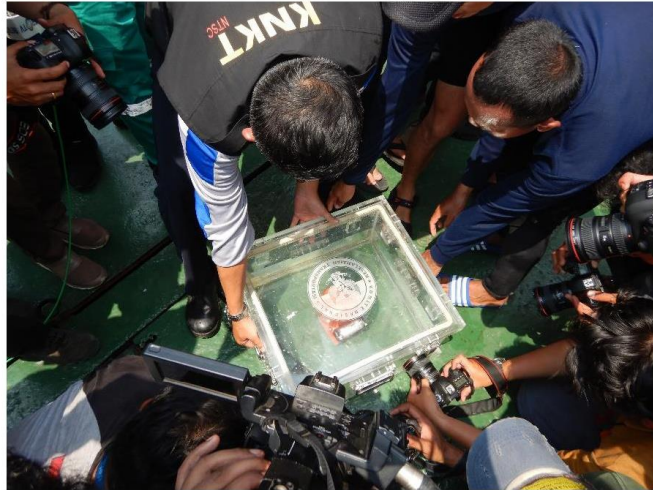
Figure 9 : The FDR CSMU transported in a fresh water contained box
