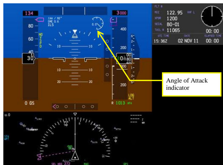
Figure 8: AOA Indicator on PFD
