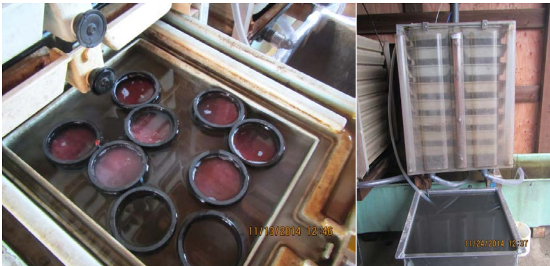
Figure 5. Embryo cups on a tray in the heath stack (left). Heath stack showing sump filled with 100% unfiltered runoff (right).
