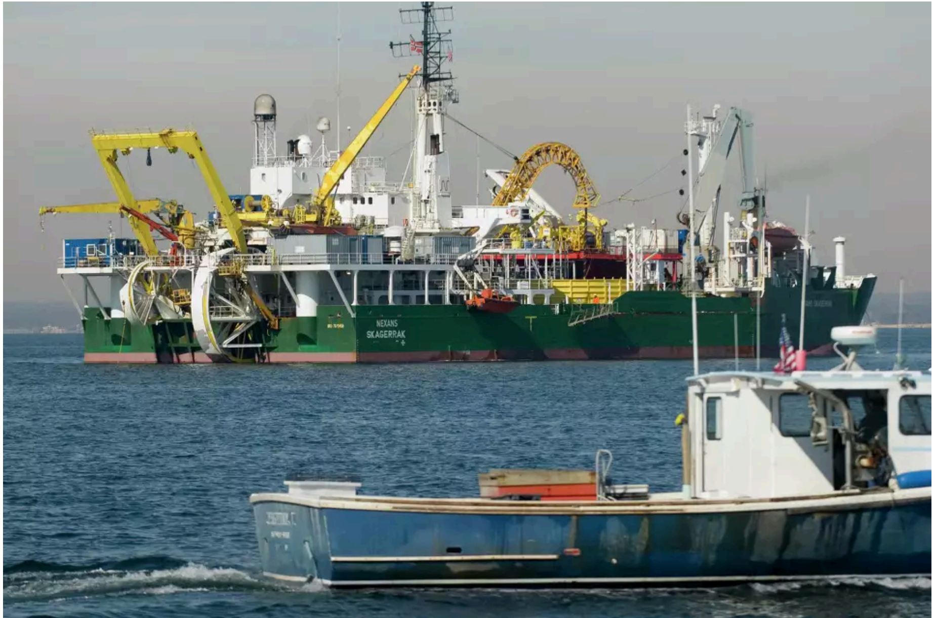
The Skagerrak lays undersea cable near the New York-Connecticut border in the Long Island Sound for Connecticut Light & Power in 2008. Undersea cables disrupt sealife and can pose environmental hazards.
