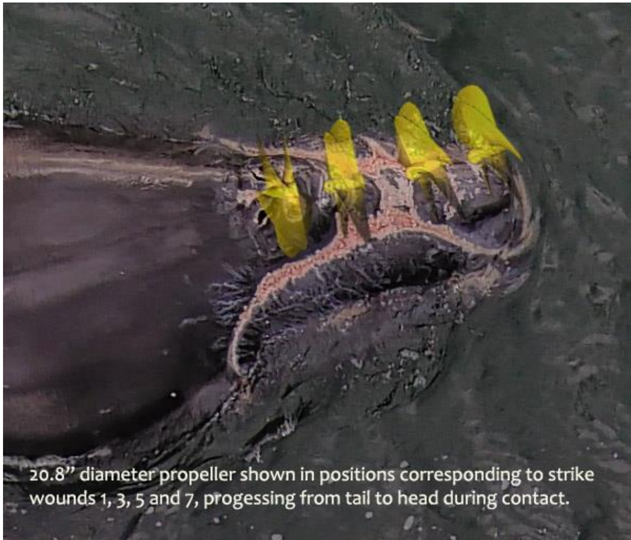
Figure 3. Illustration of the estimated propeller diameter that produced the cuts observed on the 2024 calf of Juno (Catalog #1612). An estimate of the propeller diameter was obtained using estimated measurements of calf's head length and the lengths and spacing of the cuts. The estimated propeller diameter suggests that the vessel size was between 35 and 57 feet. Credit: NOAA Fisheries, taken under NOAA permit #21371. Illustration created by forensic naval architect Paul Kamen. See NOAA Updates page for details: https://www.fisheries.noaa.gov/national/endangered-species-conservation/north-atlantic-right-whale-updates#2024-calf-of-juno-(right-whale-1612) .
