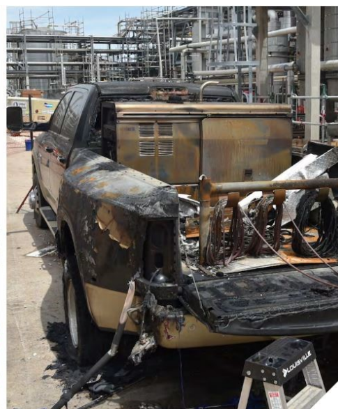
The welding machine that was the source of ignition at the Kuraray plant, where 21 workers were injured. Credit: CSB.
