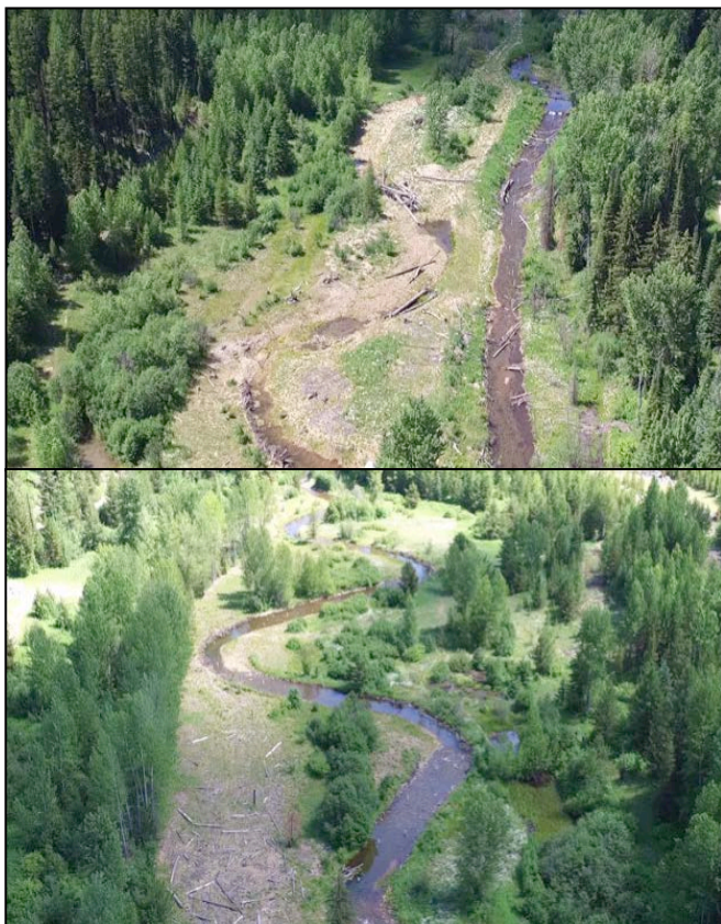
Degraded (top) and restored (bottom) reaches of Ninemile Creek. Restoration reduced channel incision, increased sinuosity and added riffle-pool sequences. Top image shows the degraded reach after overburden piles were removed, with the new, unconnected with the new, unconnected channel to the left. channel to the left.
