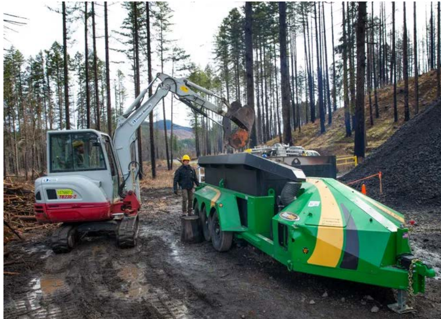
A crew loads low value excess fuels into a portable biochar machine on BLM land in Oregon. Source: The Register Guard, 2023.
