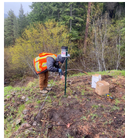
Figure 5. (below) A rain gauge being installed in a burn scar to help improve early warning to communities downstream.
