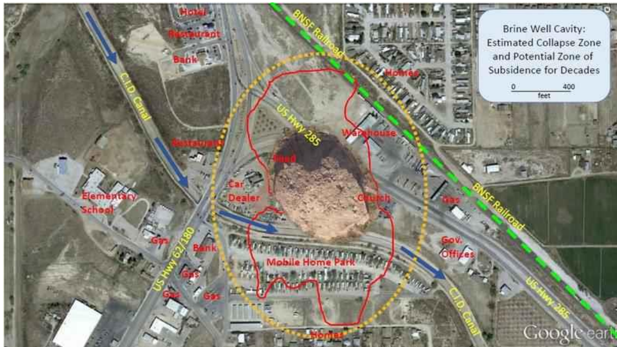
Figure 1. Image 10 showing the intersection of major roadways in the Carlsbad area that would be impacted by the formation of a sinkhole. The potential collapse zone underlies a mobile home park and poses a threat to the residents in that area (red line).
