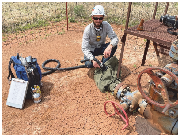
Figure 5. Emissions identified using OGI and quantified by BHFS.
