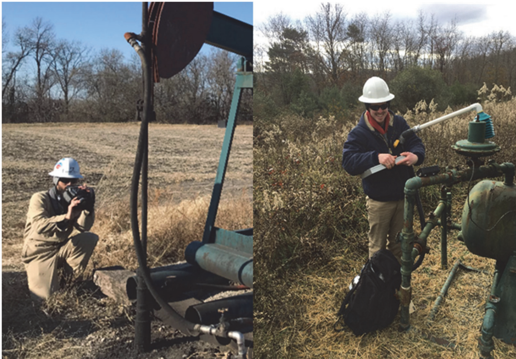
Figure A1: Direct, onsite measurements were performed with a Bacharach Hi-Flow sampler that was specially modified to allow canister samples to be drawn from its inlet.
