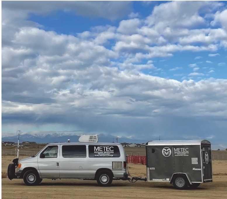
Figure A2: The CSU mobile laboratory was used to make downwind measurements using both OTM33A and dual tracer flux methods. The lab is equipped with trace-gas analyzers targeting methane, nitrous oxide, acetylene, carbon dioxide, and water vapor, and supporting instrumentation to collect weather and positioning data.
