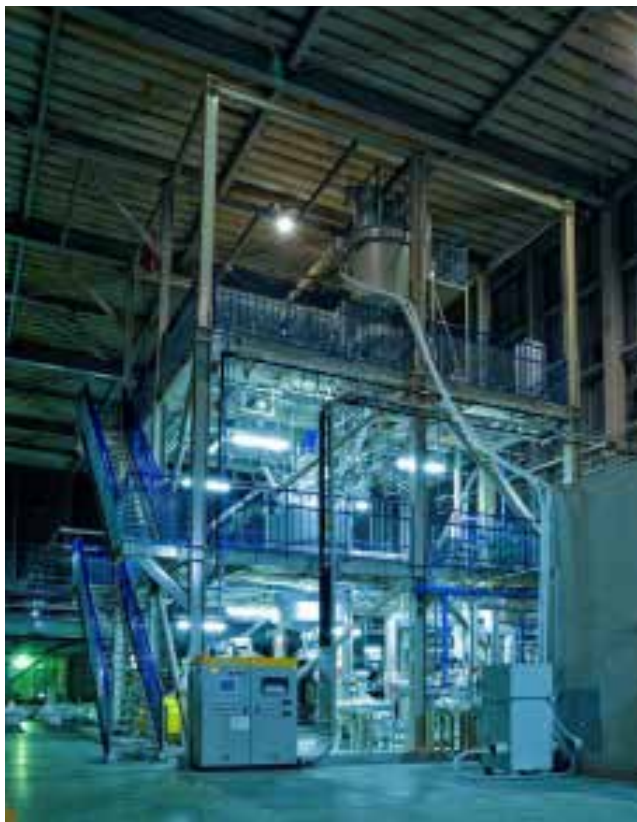
Figure 19. Panasonic pilot plant for FRP recovery. Source: Goto 2016
