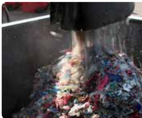
Figure 40b. Disinfected, shredded waste output from a Sanitech unit.
