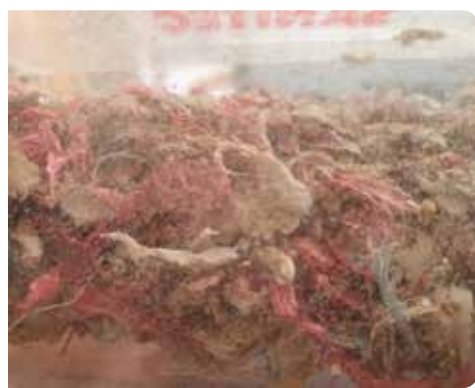
Figure 40b. Disinfected, shredded waste output from a Sanitech unit.
