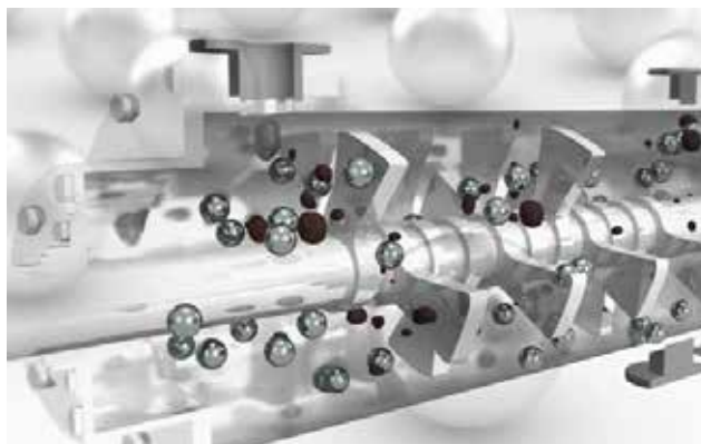
Figure 36. Illustration of the interior of a rotating ball mill. Source: EDL Asia
