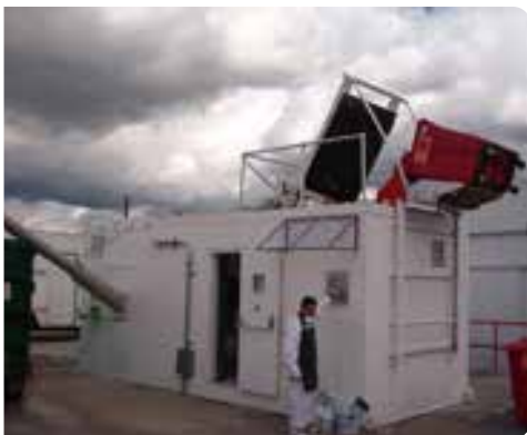
Figure 40a. Sanitech medical waste disinfection system as truck mounted and stationary units.
