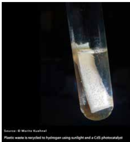
Figure 22. Photoreformation of plastic waste to hydrogen.
