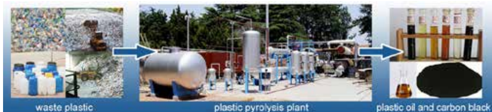
Figure 20. Plastic to fossil fuel via pyrolysis.
