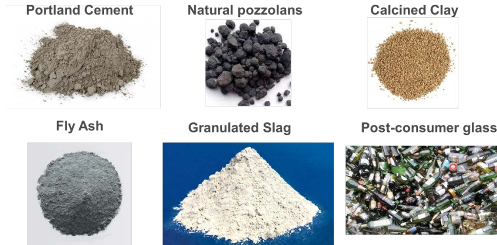
Figure 3. Examples of binders that can be used to make concrete. Binders in the top row are created from materials mined in the earth, whereas those in the bottom row are derived from waste.
