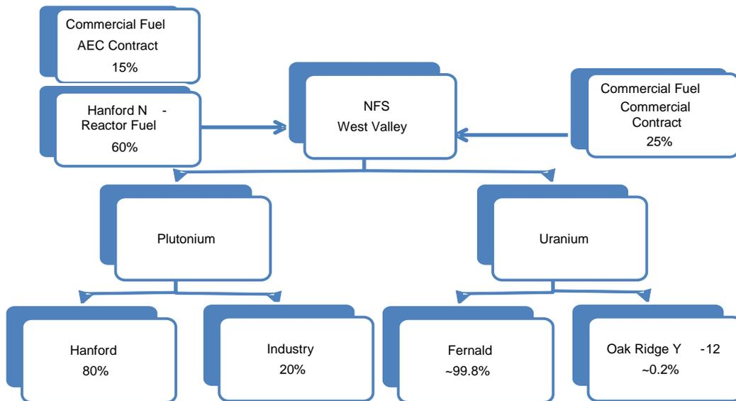
**Figure 1. Origin and Destination of the Key Materials Received and Produced During Reprocessing Operations at West Valley.**
