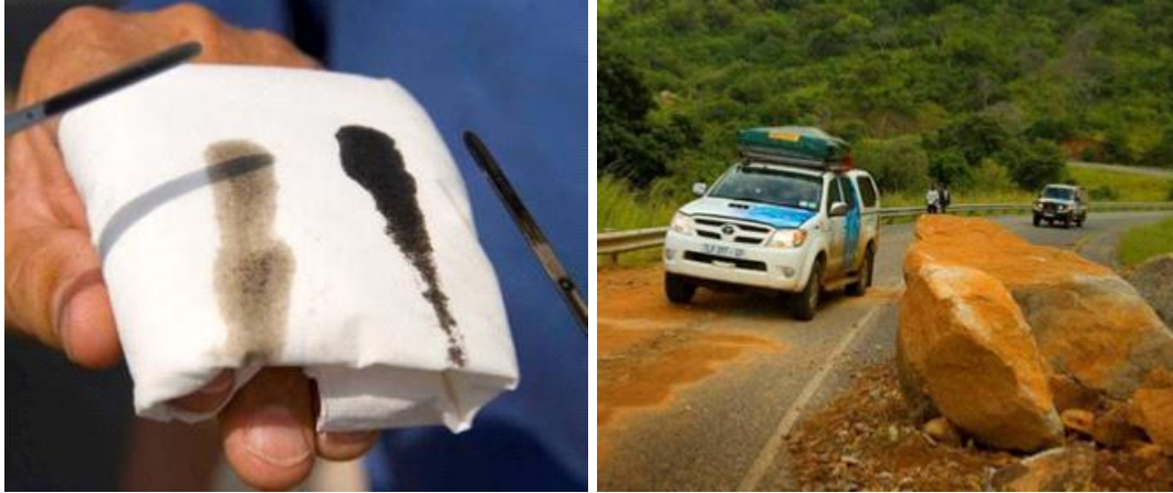
The oil from a vehicle fueled by GTL diesel, compared to the oil from an identical vehicle running on convention diesel, following an overland expedition from South Africa to Qatar.
