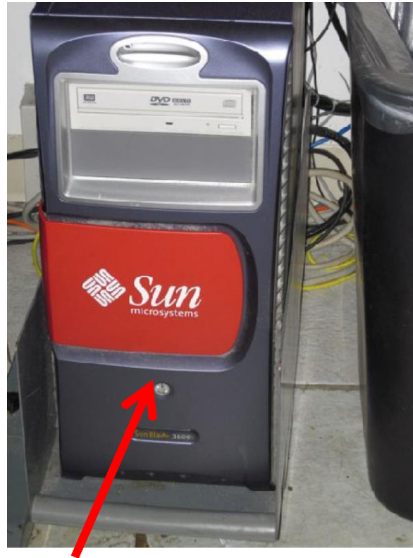
Aftermarket CPU installed on the MRI system
