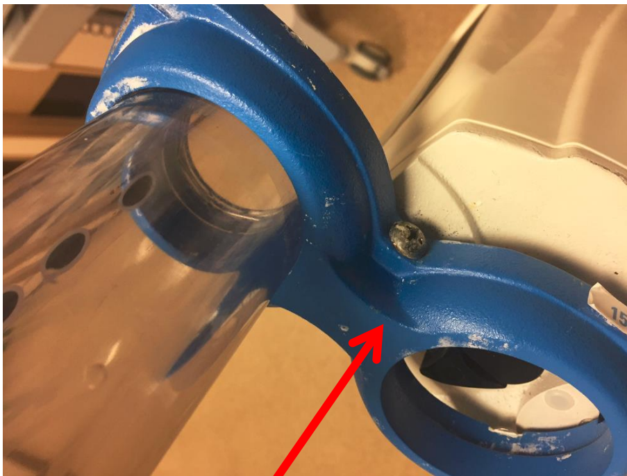
Common sheet metal screw substituted for steel pin
