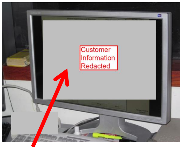
Aftermarket monitor installed on the MRI system
