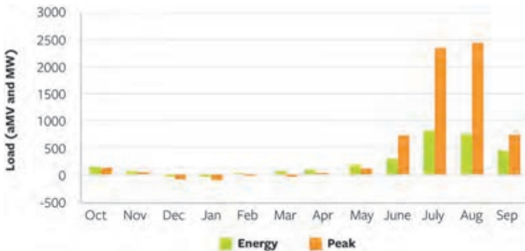
Figure 12. Projected Changes in 2035 Average and Peak Loads (NWPC 2015)
