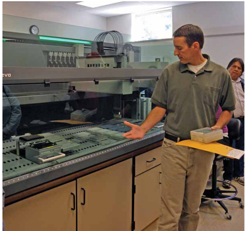
Lab Director Shawn Narum showing one of the newest pieces of lab equipment. This machine can automatically evaluate nearly 800 samples of genetic material per load.
