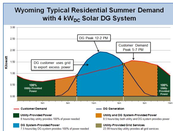
Third, utility grid services are needed 99.99% of the time to ensure power needs are met reliably and safely. The tan-shaded area along the bottom of each graph shows the utility provides all grid services 23.99 hours a day. Power is delivered through the utility's system to distributed generation customers on cloudy days, at night, when the customer's system is not
