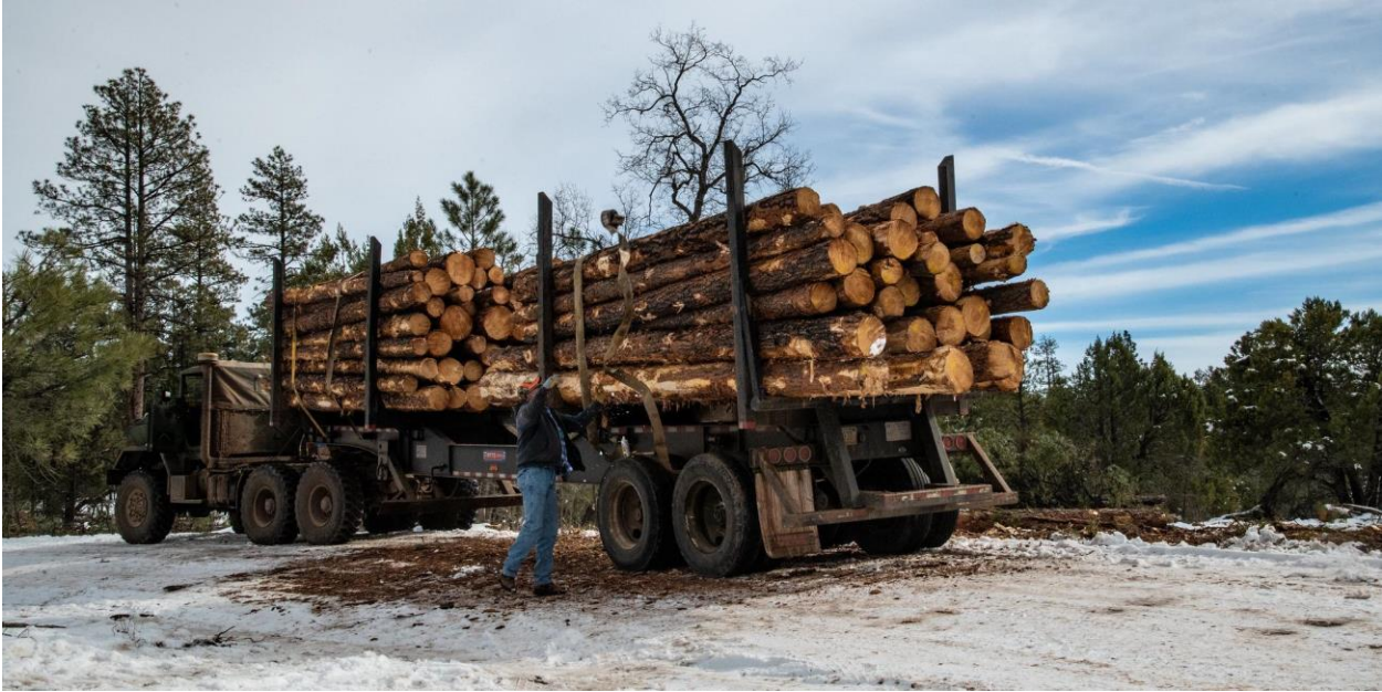
Logging truck. Photo Courtesy US Forest Service. https://www.fs.usda.gov/ . Logging trucks can haul anywhere from three thousand to six thousand board feet of timber. In 2020, the Nez Perce-Clearwater sold over eighty-four million board feet of timber. It will take over 14,000 truckloads to haul away the timber sold in 2020 once it is cut down.
