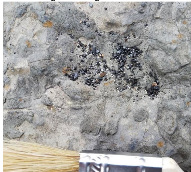
Figure 37: Same Rock, Different Date, Again Showing Accumulating Coal Particles from Railroad Bridge Over Clinch River
