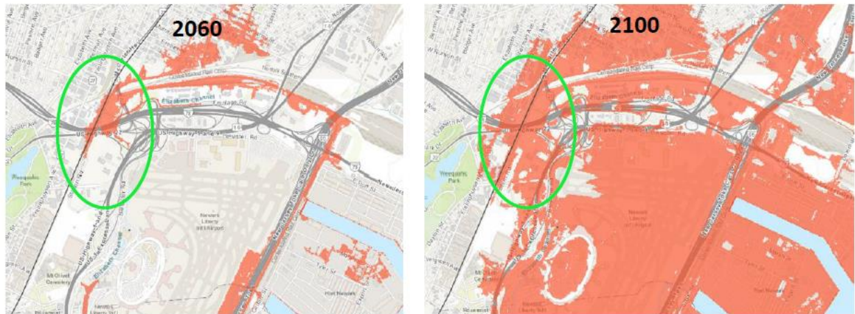
Figure 5: Amtrak rail lines in Newark, NJ exposed to chronic flooding
